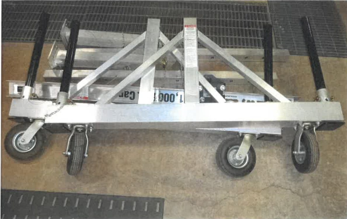
Gantry shown disassembled and ready for transport. Pieces are lightweight and manageable.
