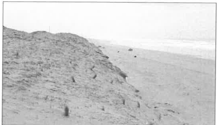
The front face of the dune mat treatment, showing poor survivorship of all but the native grass Poa macrantha . The January scarp is visible on the right.
