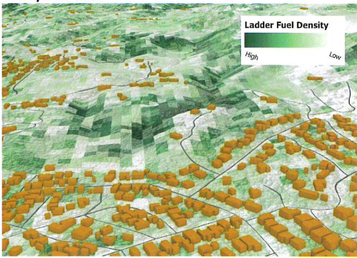
Figure X. Ladder fuel density, buildings and roads derived from lidar for Sonoma County - applications include wildfire risk mapping, vegetation management prioritization, emergency response, community health and safety
