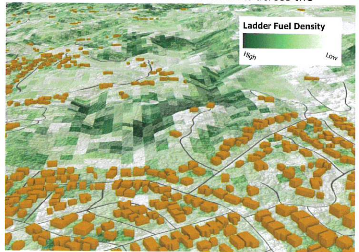
Figure 2. Ladder fuel density, buildings and roads derived from lidar for Sonoma County - applications include wildfire risk mapping, vegetation management prioritization, emergency response, community health and safety
