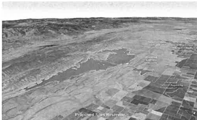
A rendering of the proposed Sites Reservoir, a 1.8 million acre-foot project that would be fed by diversions from the Sacramento River. (Image courtesy: Sites Project Authority)
