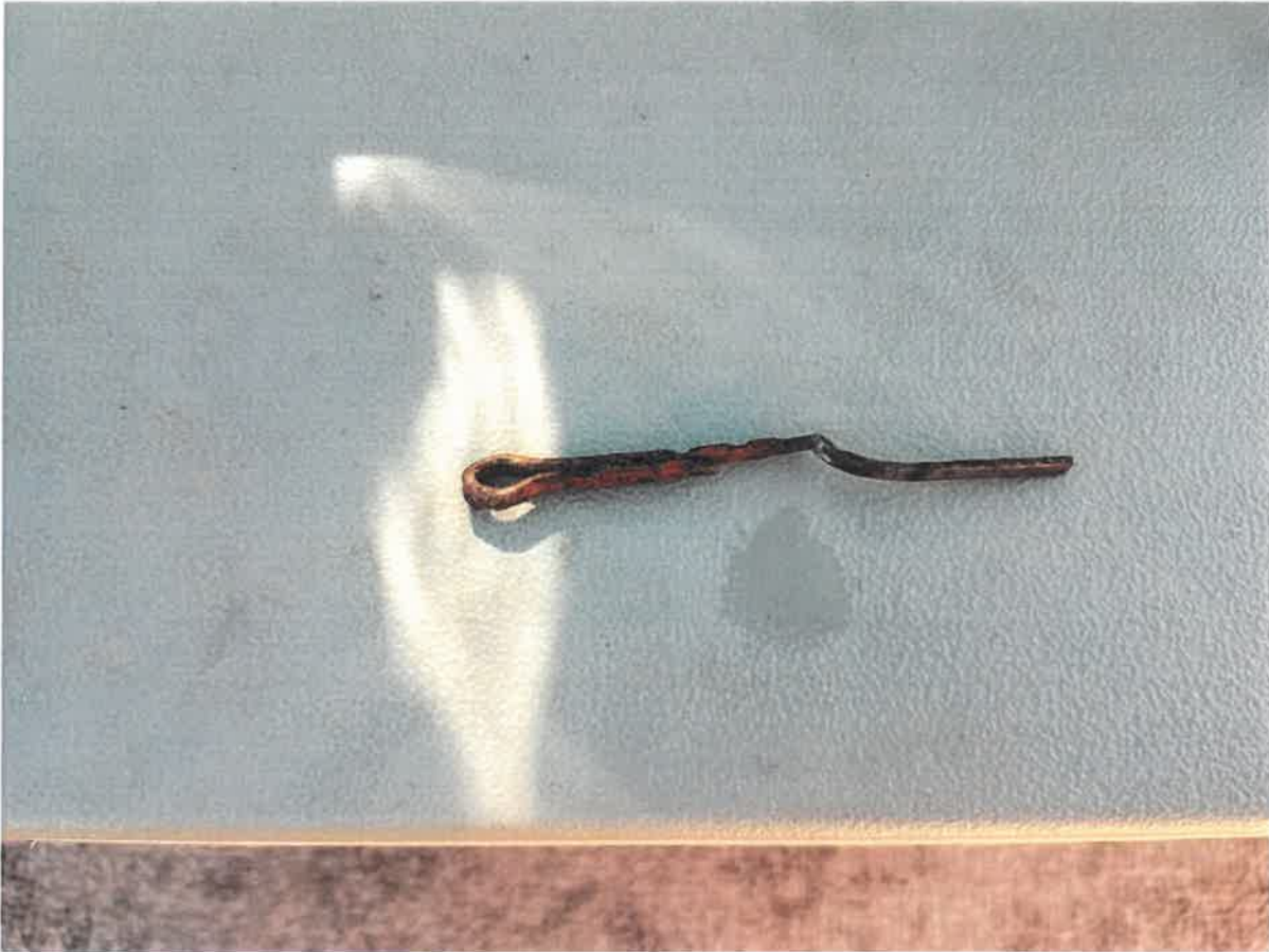
Photo 6-Original Cotter Pin Removed from West End of Boom 5
