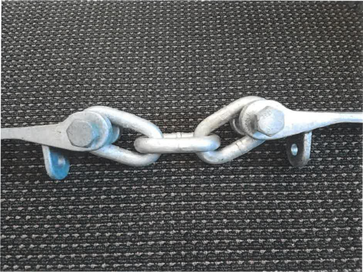
Photo 23-New Sample Boom Connection
