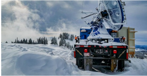
A radar truck measures precipitation during a recent cloud seeding experiment in the western United States. Joshua Aikins
