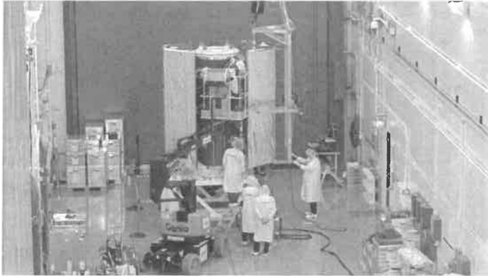
At the Harris facility at Vandenberg Air Force Base in California, one of the twin GRACE-FO satellites is integrated with the multi-satellite dispenser structure that will be used to deploy the satellites during launch on the SpaceX Falcon 9 launch vehicle. Launch is scheduled for May 19. Credit: Airbus
